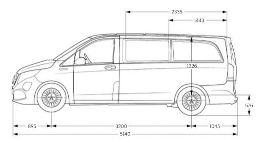
All figures in millimetres. The pictured dimensions are mean values. They are valid for vehicles with standard equipment and in unladen condition.
