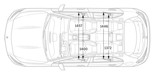
All figures in millimetres. The dimensions shown are mean values. They are valid for vehicles with standard equipment and in unladen condition.
